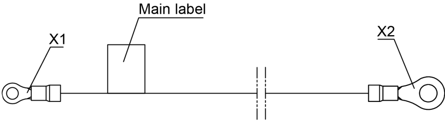
Figure 6-2 Structure of a ground cable
